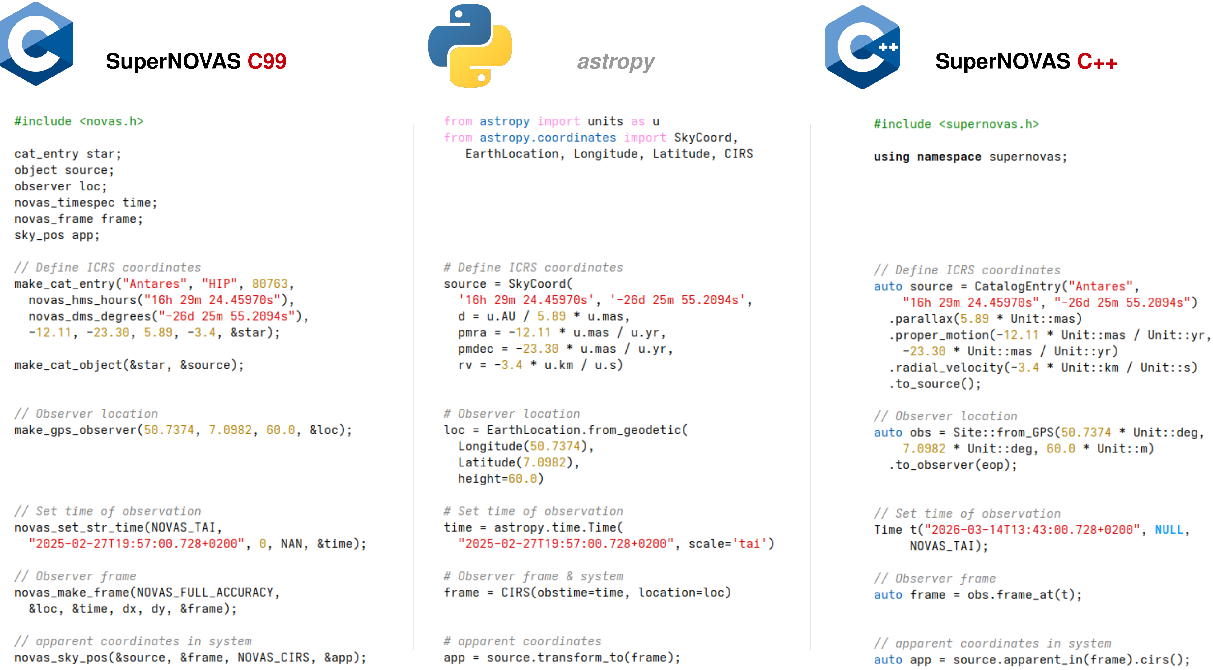
Fig. 2: Calculating the position of a star in the Celestial Intermediate Reference System (CIRS) of date.
