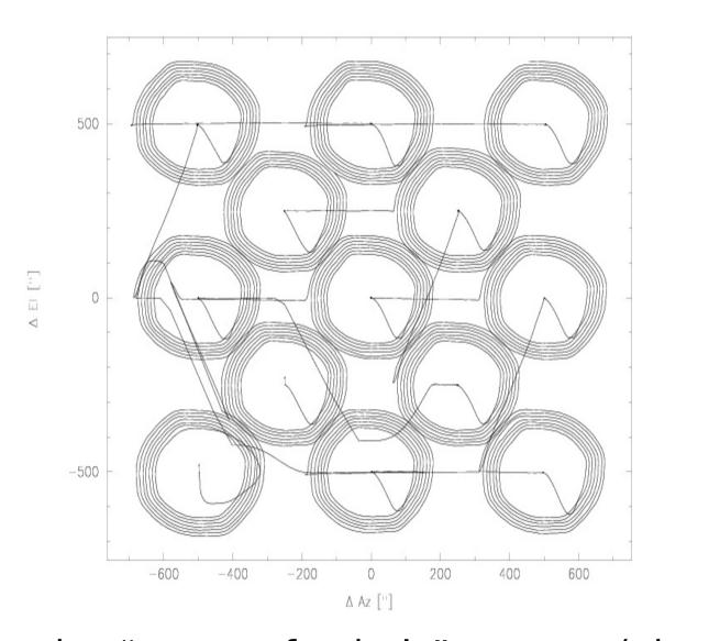
We used a "raster of spirals" pattern (above) to achieve uniform coverage over a 0.5 deg  $\times$  0.5 deg area (see below). Total power bolometer arrays, like LABOCA, require fast, cross-linked scanning patterns for optimal imaging under a bright, fluctuating atmospheric background and other instrumental noise sources. When used correctly, this technique yields images that are far superior to the traditional chopped or jiggle mapping modes.
