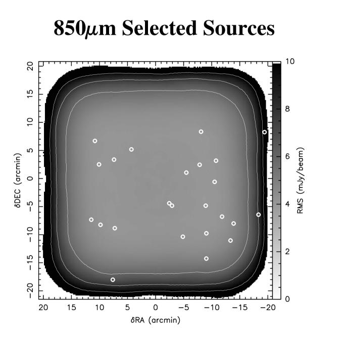
The noise map (above) with the positions of the sources extracted (see source list below) indicated as circles. Contours are shown at 2, 4, and 6 mJy/beam rms levels. Upon completion of the project, we hope to reach  $\sim 1$  mJy/beam sensitivities in the same area, making our survey deeper and covering a larger area than any preceding deep submm survey.
