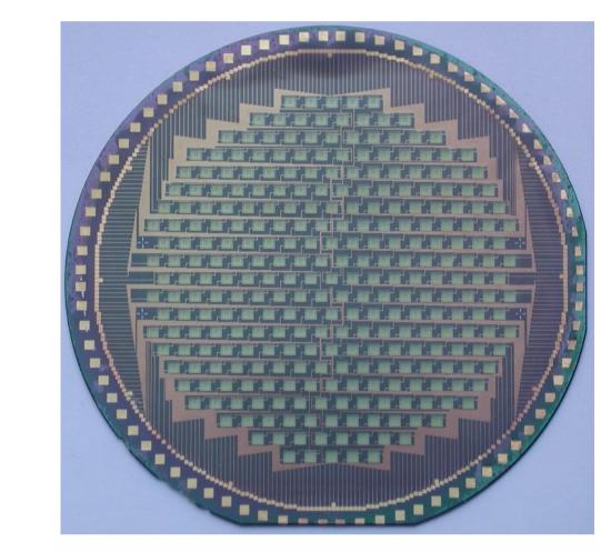
LABOCA (E. Kreysa & G. Siringo) with its 295 pixels is the ideal instruments for sensitive mapping of large fields (shown is a picture of the detector array above). It is capable of downintegrating approximately 10 times faster than the highly successful SCUBA
